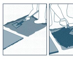
Remove the turf and dig out about 5 cm of soil.
