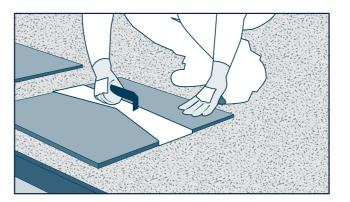
Position the tile and then compact the edges in order to level the tile with the substrate. It is suggested to use a joint of at least 4 mm to allow good water drainage.
