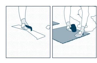
Lay the tile, so as to have an approximately 0.5 cm level difference, between the tile and the ground.
