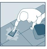
Once the installation is finished grout the flooring. Remember to observe the times indicated by the manufacturer for light foot traffic before walking on the tiles. "Post-installation" cleaning is mandatory at the end of the work and is required to remove residues
