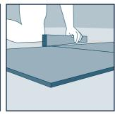
Check the planarity of the flooring regularly during the laying operations.
