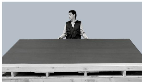
1 | 100x300 cm and 120x260 cm slabs of Kerlite can be lifted by one person. Lift the slab with open hands. Slowly raise the longer side so as to eliminate the suction effect, due to contact with the underlying slab, and ensure a good grip. When handling the use of gloves is recommended.
