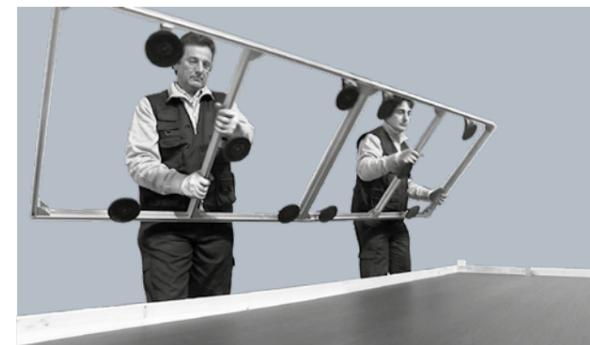
4/5 | 100x300 cm and 120x260 cm slabs of Kerlite can be handled by two people with the help of a special frame. Fix the frame to the slab when it is still on the pallet. Raise the frame and slab to eliminate the suction effect.
