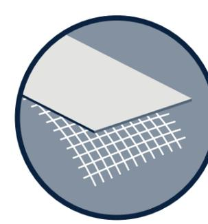
fibreglass mesh on the **rear of the slab**
